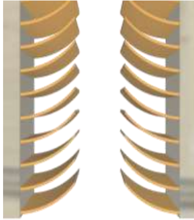
Fig 11. Diagram illustrating inwards angling of rubber strips
