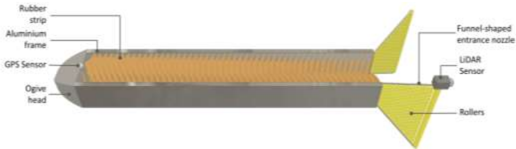
Fig 2. Labelled diagram of AUV recovery cradle
