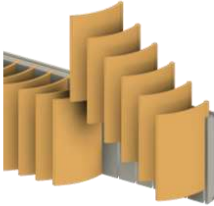
Fig 12. Diagram illustrating removable aluminium frame
